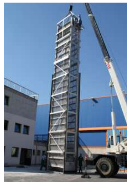
→ GNAFO1 dual flow belt screen, factory testing
