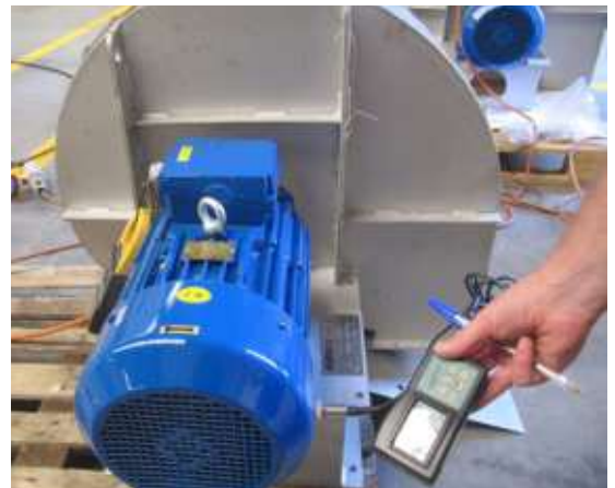
→ Centrifugal fan (aspirator) for odour control
