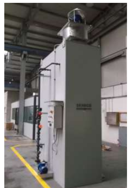
→ Air scrubber for H 2 S abatement
