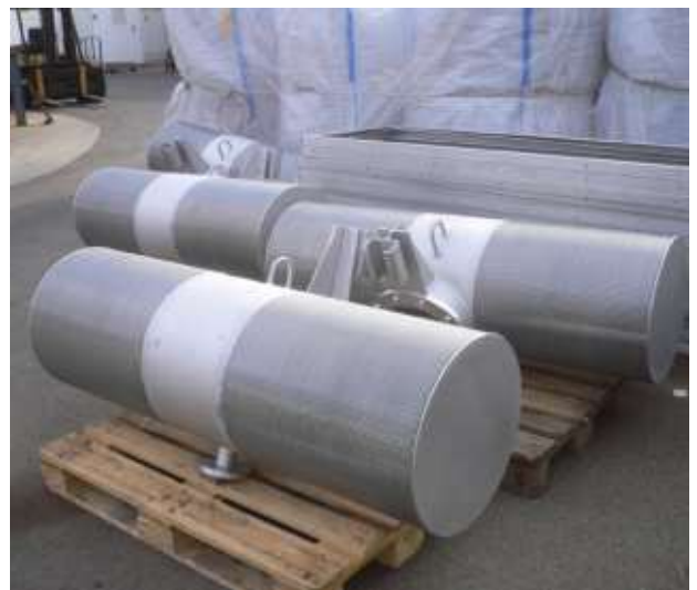
➔ T-shaped water intake ITC
